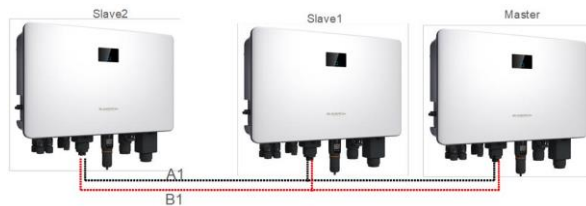
Figure 1-2 Master-slave inverter communication wiring
